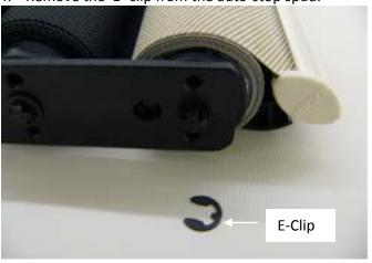
NOTE: Only remove the E-Clip from the Auto-Stop that you are adjusting. Removal of the E-Clip from the shade spring may allow the spring to lose tension.
